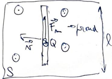
$$U = \frac{W}{q} = \frac{F_m l}{q} = \frac{q(\vec{v} \times \vec{B})l}{q} = vBl$$
