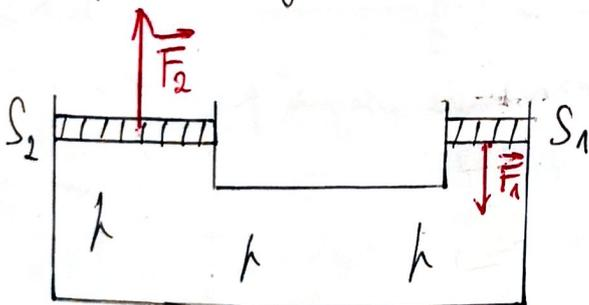
$$p = \frac{F_1}{S_1} = \frac{F_2}{S_2} \Rightarrow \frac{F_1}{F_2} = \frac{S_1}{S_2}$$
