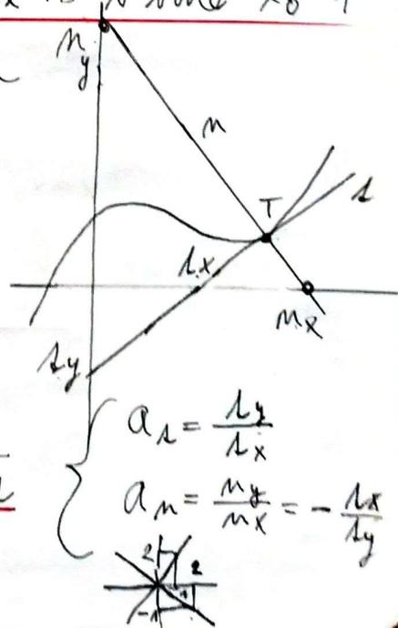
$$a_m = -\frac{1}{a_L} \quad \left\{ \begin{array}{l} a_L = \frac{k_y}{k_x} \\ a_m = \frac{m_y}{m_x} = -\frac{k_x}{k_y} \end{array} \right.$$
